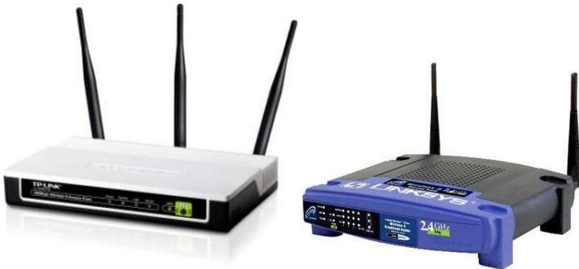
Above: examples of a wireless-N access point (AP). An AP can be connected by a long Ethernet cable to your B4RN router to provide strong broadband in areas of your house with poor WiFi signal..
